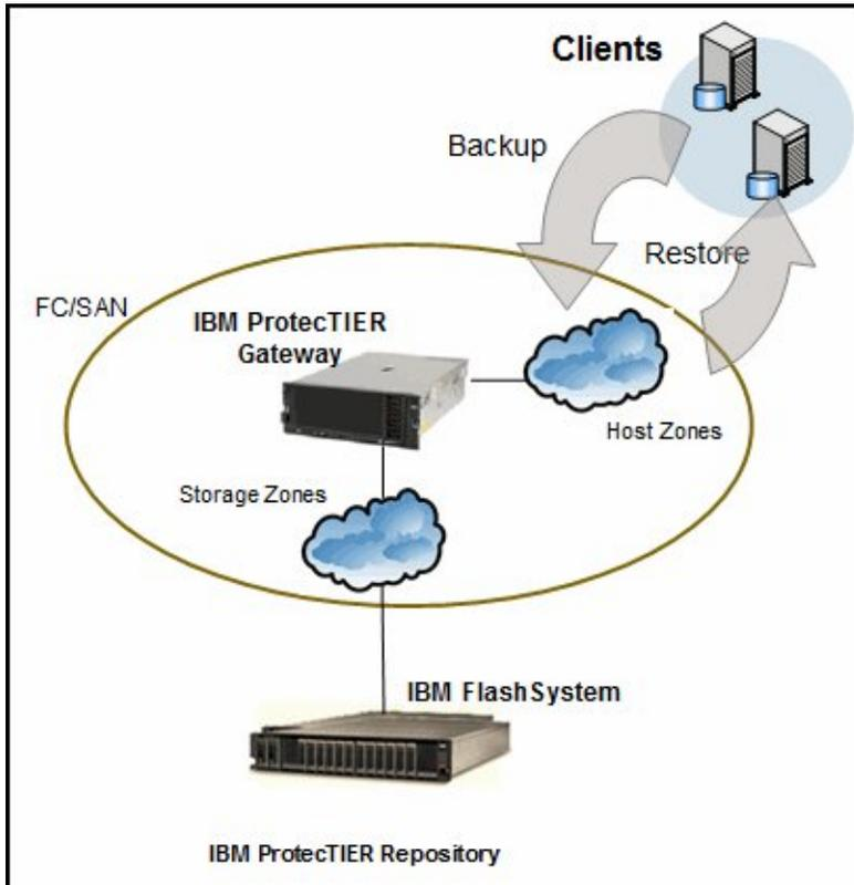
Figure 2. IBM FlashSystem and ProtecTIER architectural overview
