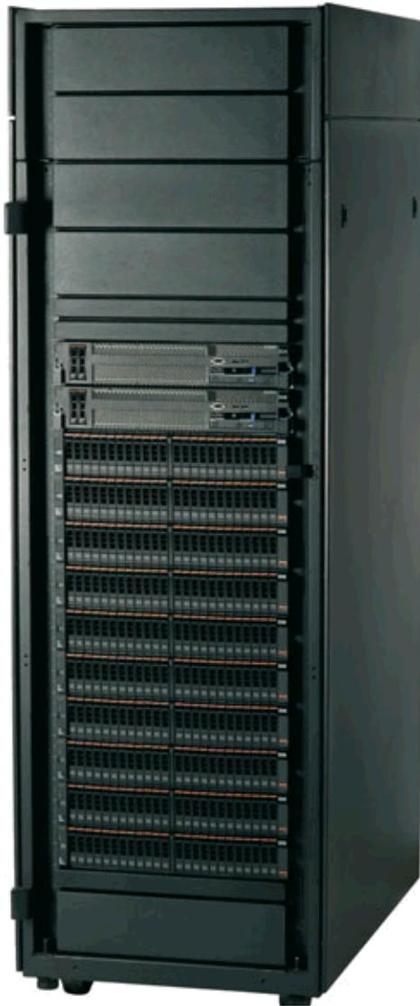
Figure 5 Storwize V7000 Unified with nine disk expansion enclosures, each with twenty-four 2.5-inch drives
