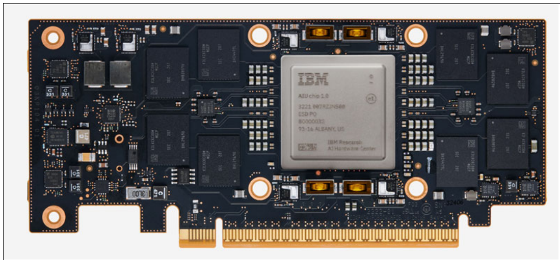
Figure 4-6 IBM Power AI Acceleration Chip on 75W PCIe Adapter with 128 GB LPDDR5 Memory.
