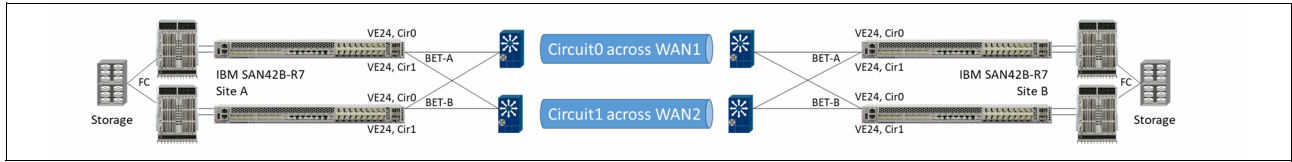
Figure 8-4 Dual fabric FCIP architecture extending production fabric
