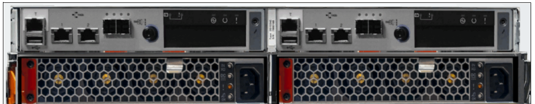
Figure 1-47 Rear view of an IBM FlashSystem 5035
