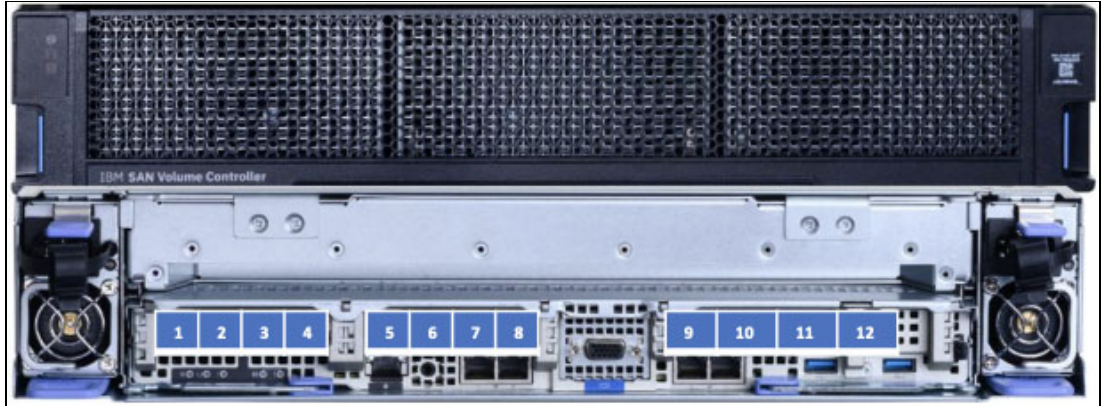
Figure 2-10 SV2/SA2 node layout
