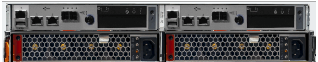
Figure 1-50 Rear view of an IBM FlashSystem 5045
