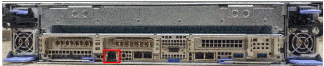
Figure 3-7 Technician port IBM SAN Volume Controller 2145-SV2
