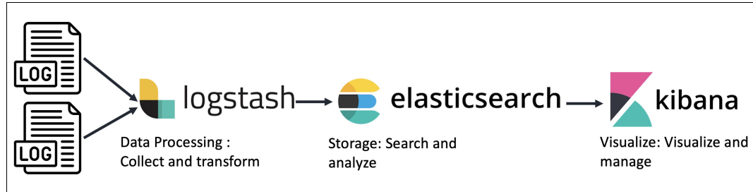
Figure 8-6 Classic ELK stack architecture
