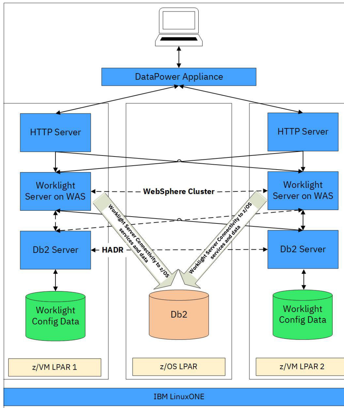
Figure A-2 Access from a mobile device to a back-end transactional core system
