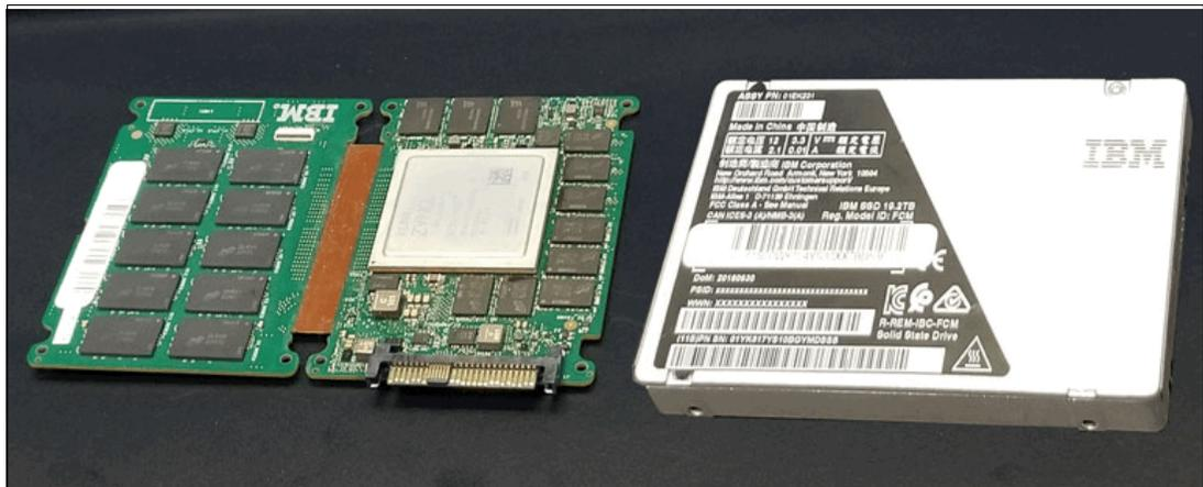
Figure 7 IBM FlashCore Module (NVMe)
