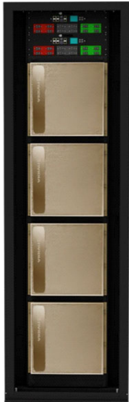
Figure 2-3 Compute rack that is configured with 4x DGX B200 nodes
