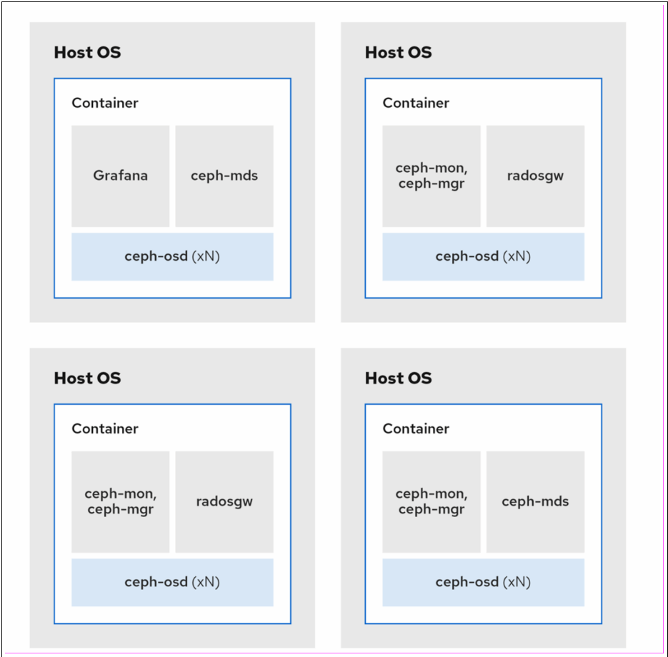
Figure 4-4 Example of service colocation for a four-node cluster
