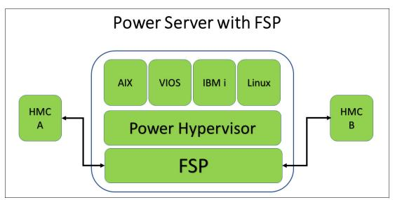
Figure 2-2 FSP-based Power server
