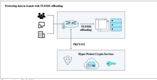
Figure 8-21 shows how TLS and SSL can be managed.
