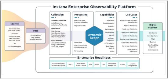
Figure 7-2 provides an overview of the IBM Instana Enterprise Observability Platform.
