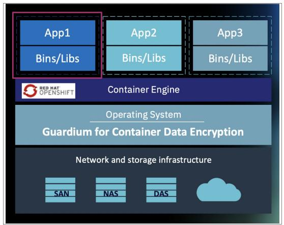
Figure 6-5 IBM Security Guardium for Container Data Encryption
