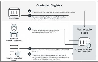
Figure 3-5 Hacker attack on a poorly configured Docker server<sup>6</sup>
