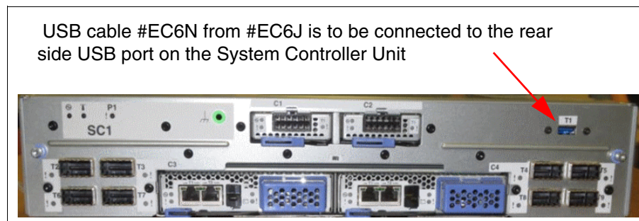
Figure 2-22 Rear view of the SCU showing the USB port for connection
