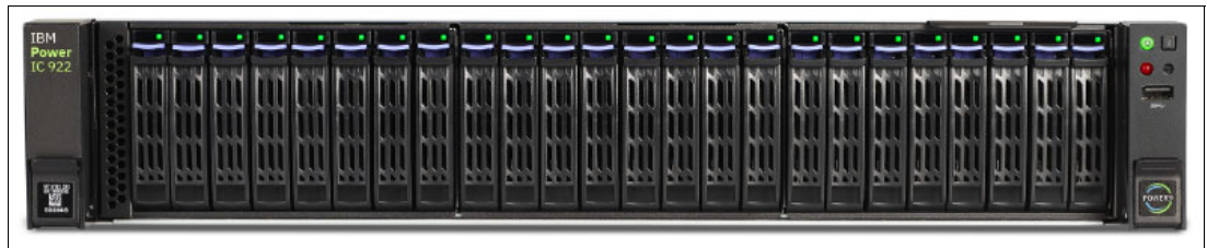
Figure 1-2 Front view of the Power IC922 server
