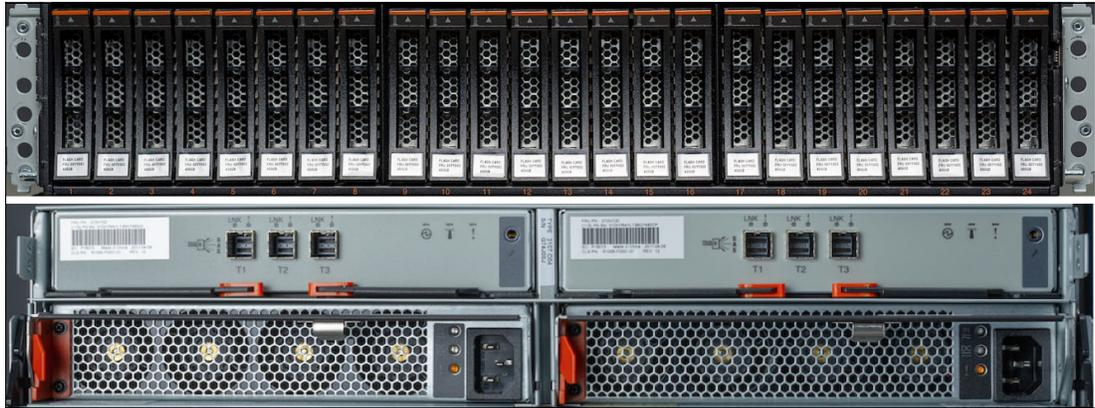
Figure 5 HPFE Gen2 front (top) and rear (bottom)
