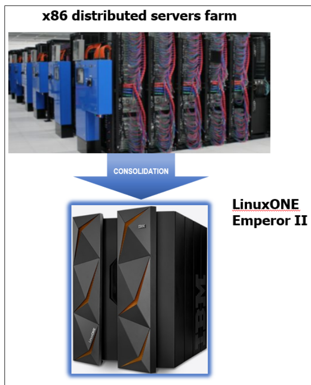
Figure 1-7 x86 scale-out infrastructure consolidated to a single LinuxONE machine
