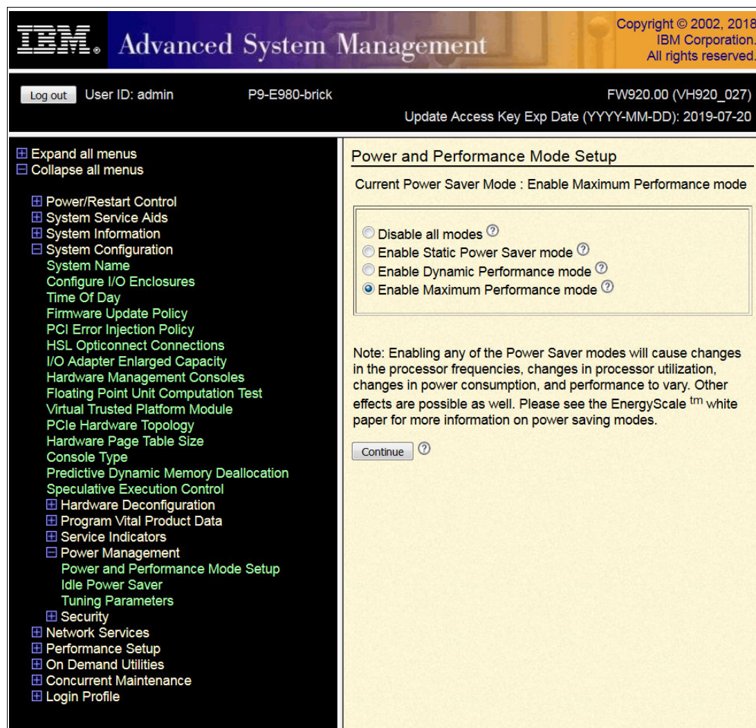
Figure 2-10 Power E980 ASMI menu for power and performance mode setup
