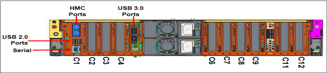
Figure 2-10 Rear view of a rack-mounted Power H922 system with PCIe slots location codes
