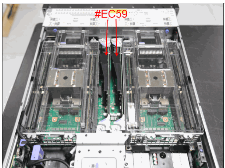
Figure 2-10 Two #EC59s in a Power L922 server
