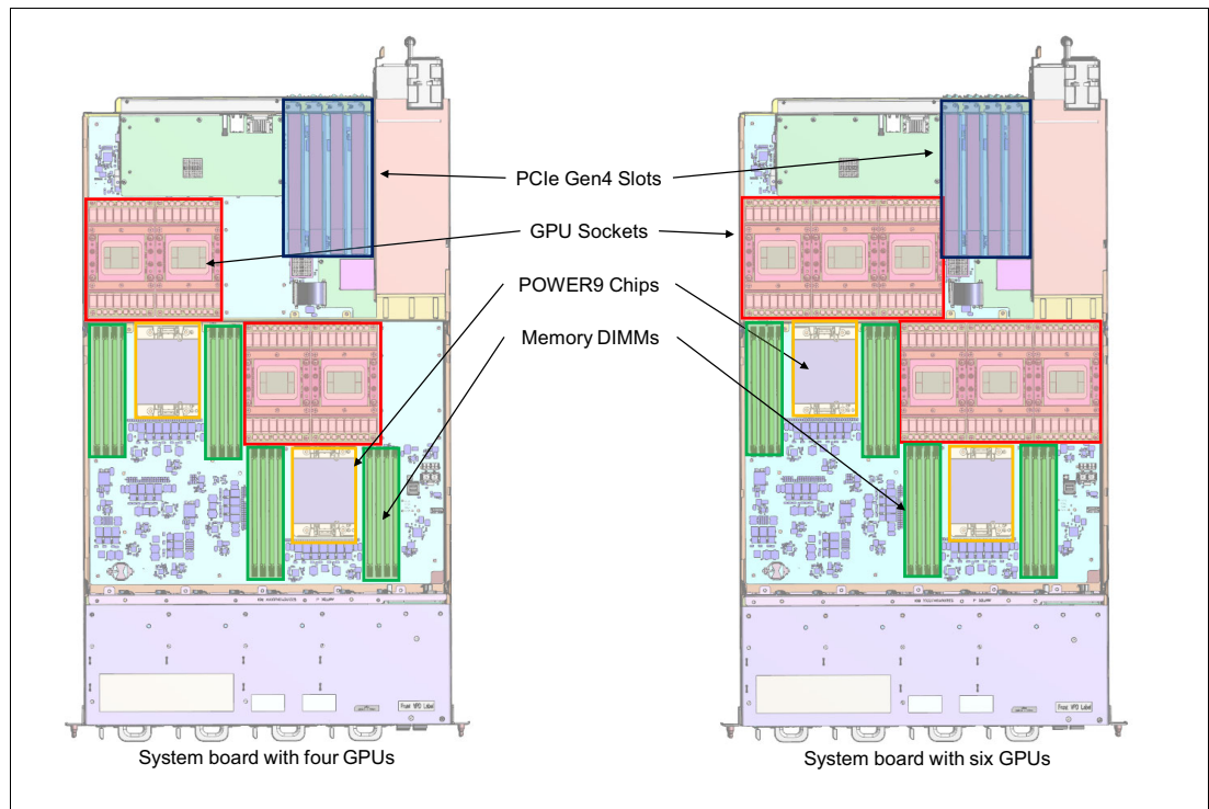
Figure 2-1 Component location for 4-GPU and 6-GPU system board
