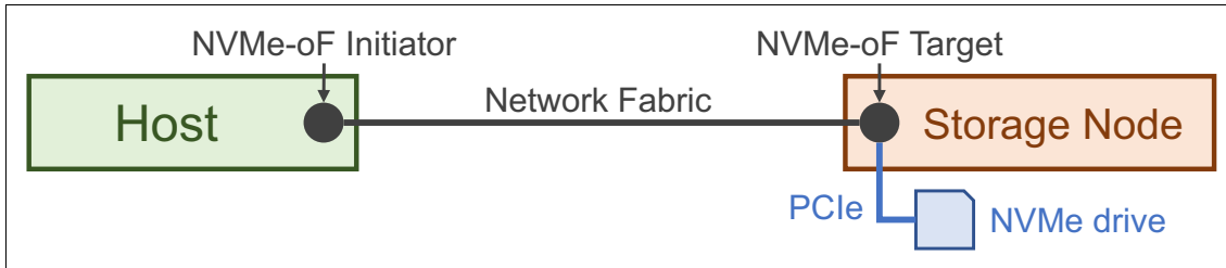
Figure 3 Simple NVMe over Fabrics topology
