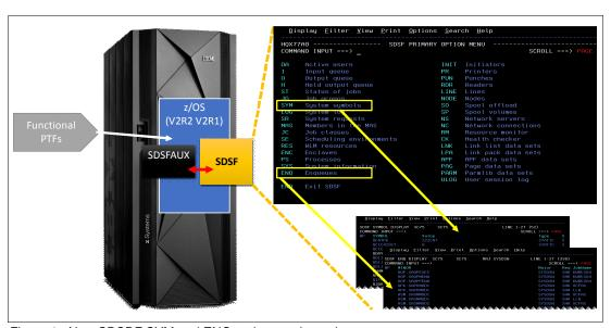
Figure 1 New SDSDF SYM and ENQ options and panels
