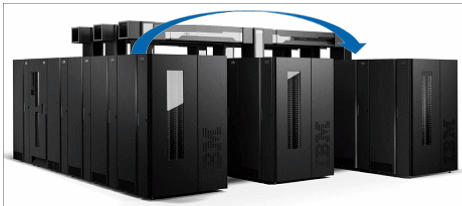
Figure 4-3 TS3500 Shuttle Complex moves tapes cartridges between physical libraries
