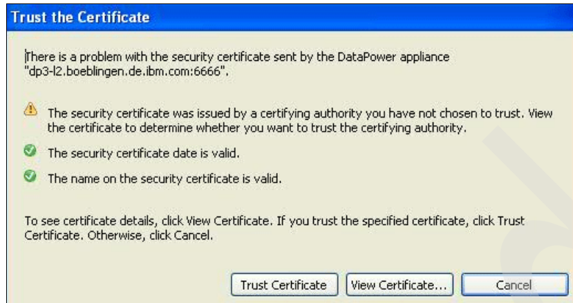
Figure 14 The Trust Certificate window is displayed when an appliance is first contacted
