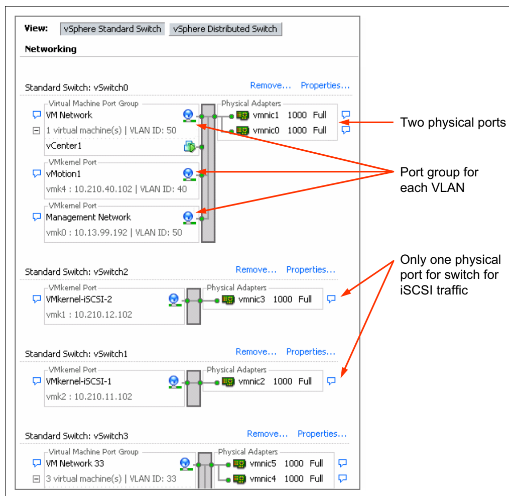
Figure 3-4 Network configuration in vSphere ESXi virtual Ethernet switches and ports
