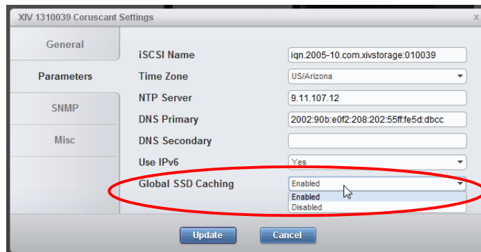
Figure 6-5 System settings for Global SSD Caching
