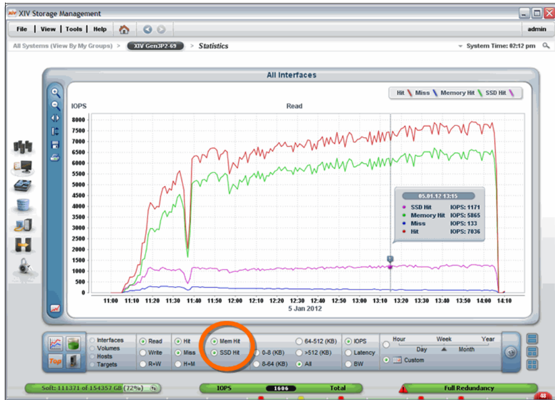
Figure 7-1 Mem Hit and SSD Hit parameters
