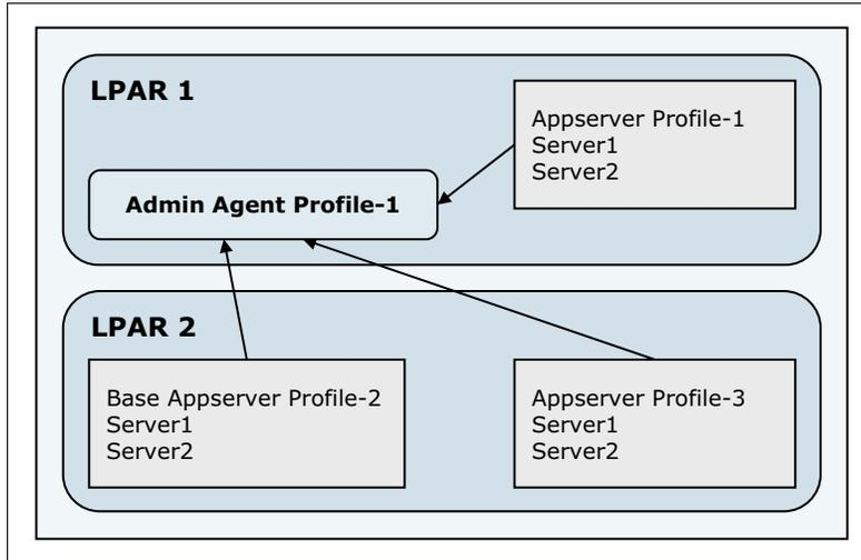
Figure 6 z/OS system with a cross-registered LPAR
