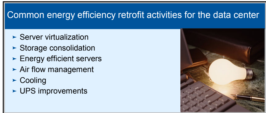
Figure 6 There are many ways to save energy in most existing data centers
