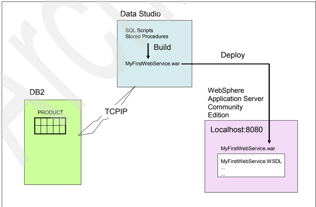
Figure 40 Overview picture of build and deploy
