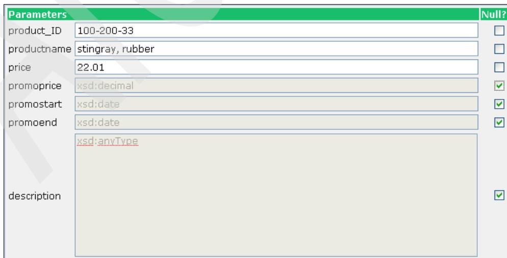
Figure 74 Use of Test Client to insert NULL values with REST
