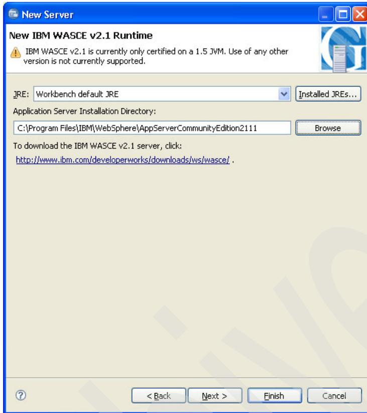
Figure 35 Configuration of a new WASCE Runtime
