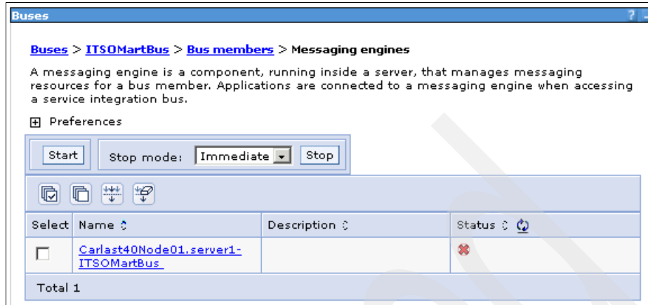
Figure 2 Checking the messaging engine status
