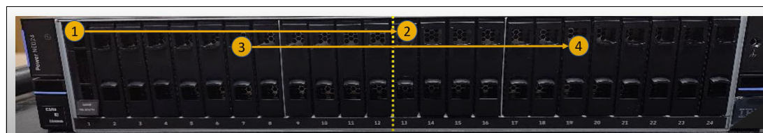
Figure 3-18 Drive installation order
