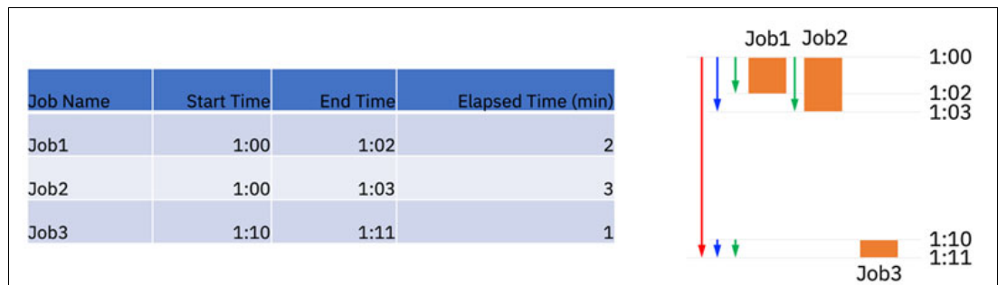
Figure 5-6 Batch application with sample jobs running example
