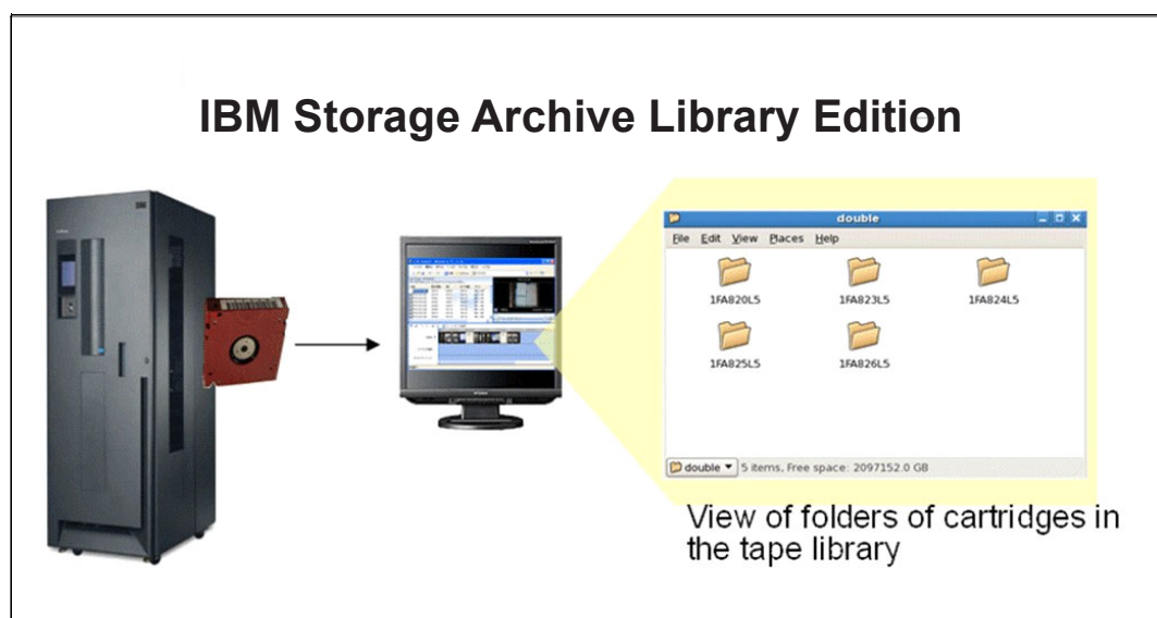
Figure 3-3 IBM Storage Archive LE view of tapes as folders
