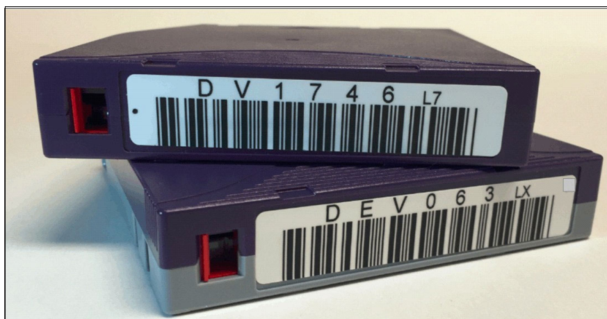
Figure 2-3 LTO 7 data cartridge (purple) and WORM cartridge (purple with platinum bottom)
