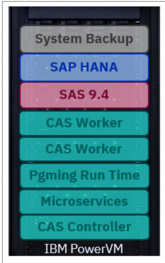
Figure 3-5 MPP mode: Scale-up multi-partition
