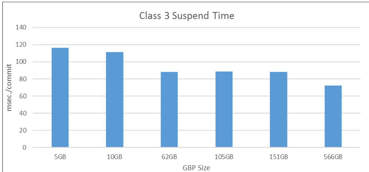
Figure 3-20 Class 3 suspension time with increasing GBP sizes
