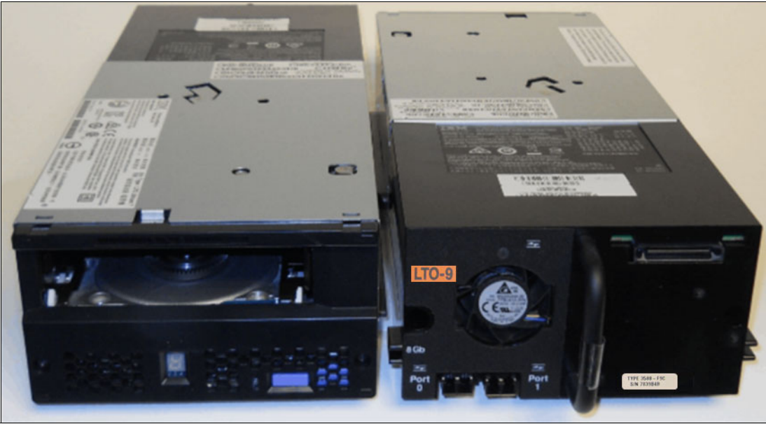
Figure 2-19 LTO Ultrium 9 (3588 F9C) tape drive
