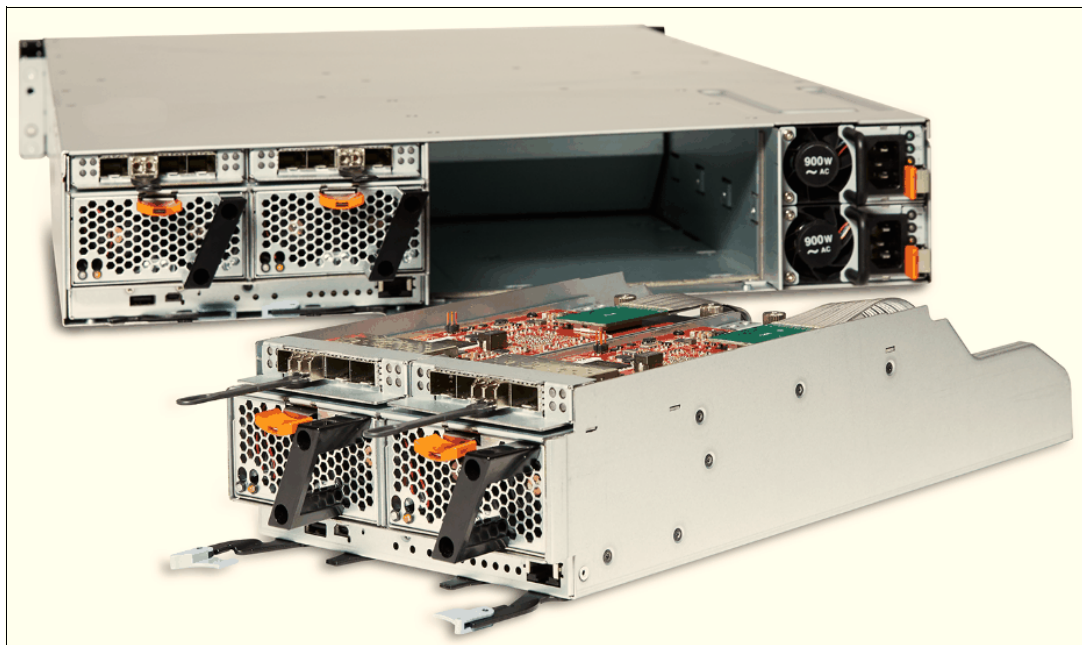
Figure 2-6 Rear view of the FlashSystem 840 with canister removed
