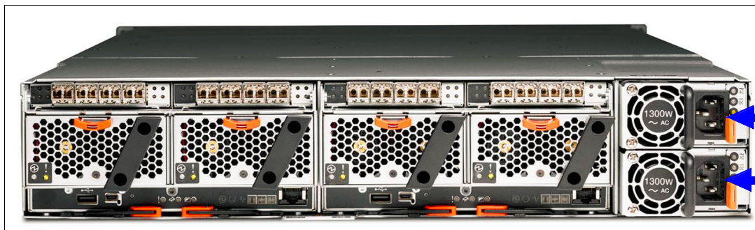
Figure 3-1 FlashSystem 840 rear view and power connections
