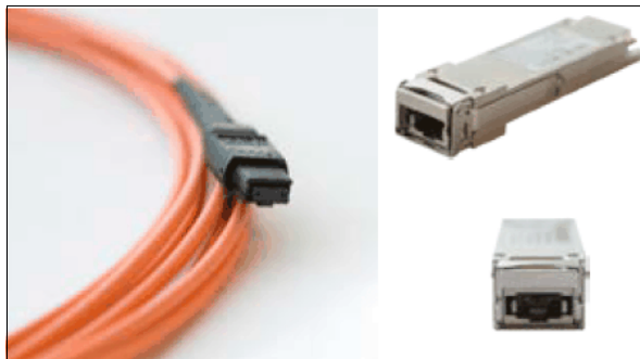
Figure 2-28 UltraScale ICSL cable and QSFP
