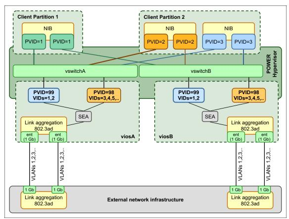
Figure 4-1 Dual Virtual I/O Server configuration with two virtual switches
