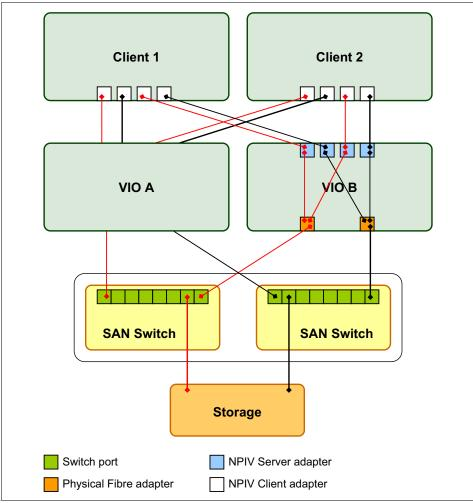
Figure 5-4 NPIV configuration with dual Virtual I/O Servers
