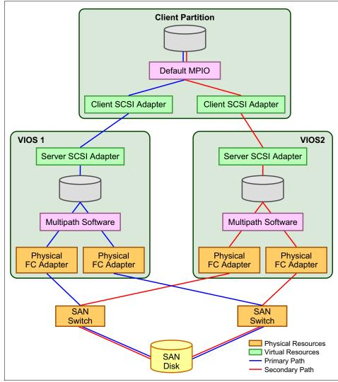
Figure 5-1 Virtual SCSI client with multipathing from dual Virtual I/O Servers
