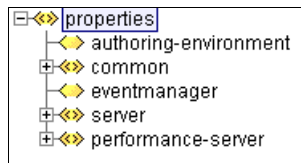
Figure C-4 Performance Data Warehouse (PDW) configuration XML file structure
