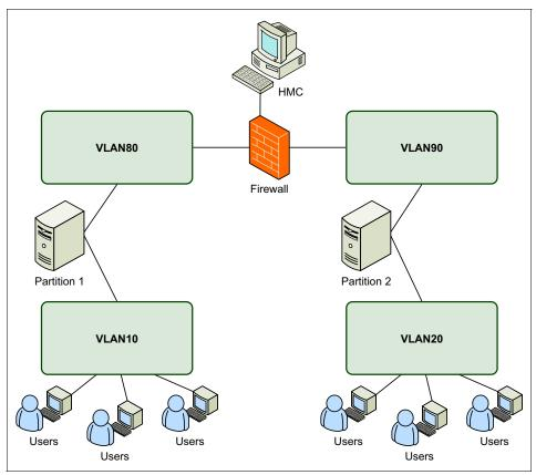
Figure 16-72 Cross-network VLAN tagging with a single HMC
