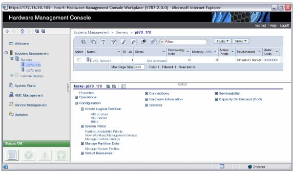
Figure 12-19 shows the created Virtual I/O Server partition on the HMC.
