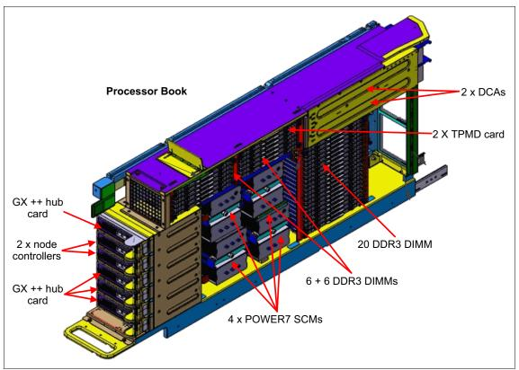
Figure 3-3 shows the layout of a processor book and its components.
