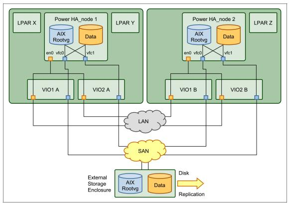
Figure 7-3 Live Partition Mobility capable virtualized environment diagram
