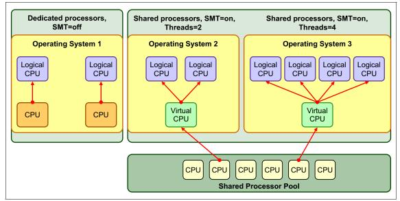
Figure D-1 Physical, virtual, and logical processors
