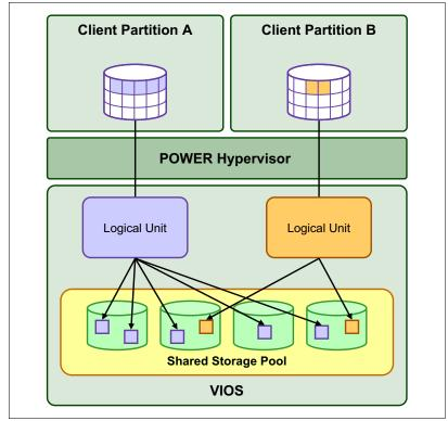
Figure 4-8 Thin-provisioned devices in the shared storage pool
