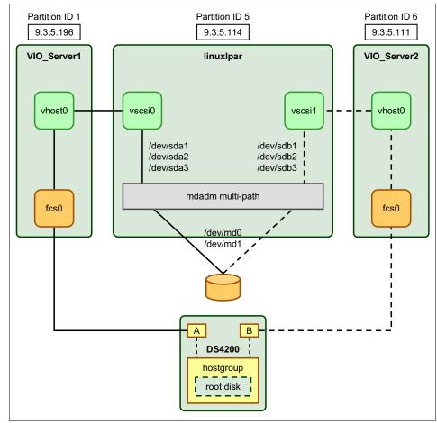
Figure 16-38 Linux client partition using MPIO to access SAN storage
