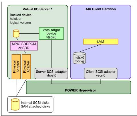
Figure 10-16 Using MPIO with IBM System Storage DS8000
