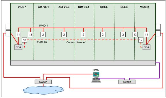
Figure H-2 shows the basic layout of partitions and the slot numbering of virtual Ethernet adapters.
