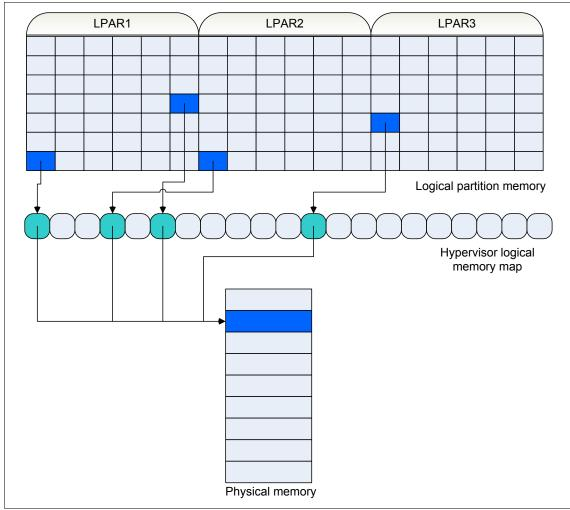
Figure 3-1 Memory structure with Active Memory Deduplication enabled
