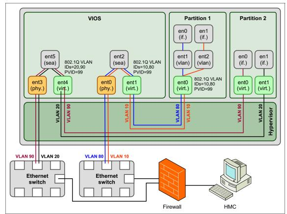
Figure 16-71 HMC in a VLAN tagged environment
