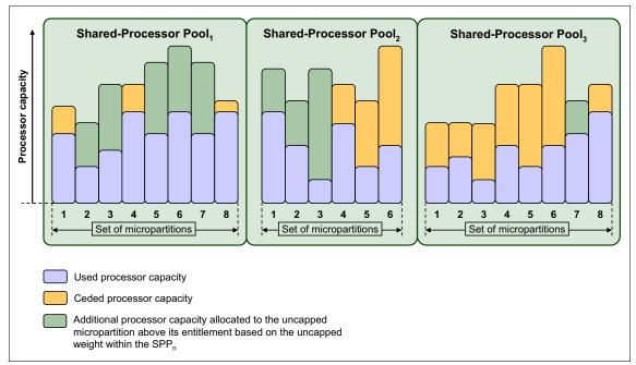
Figure 8-2 Example of Multiple Shared-Processor Pools
