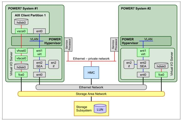
Figure 11-3 Hardware infrastructure enabled for Live Partition Mobility
