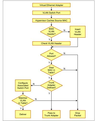
Figure 10-21 shows a graphical representation of the behavior of the virtual Ethernet when processing packets.
