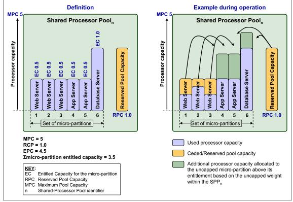
Figure 8-6 Web deployment using Shared-Processor Pools
