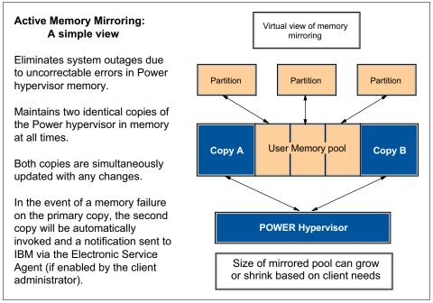
Figure 3-2 A simple view of Active Memory Mirroring
