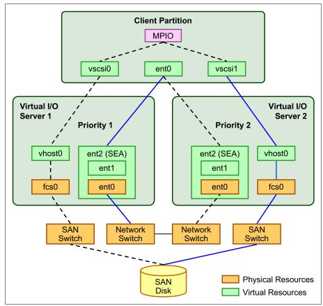
Figure 10-3 Separating disk and network traffic
