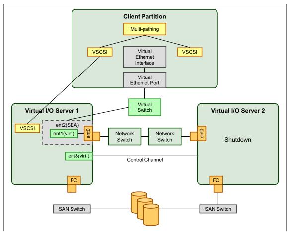
Figure 10-2 Redundant Virtual I/O Servers during maintenance
