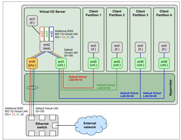
Figure 16-68 VLAN configuration scenario
