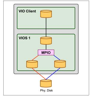
Figure 4-14 Single Virtual I/O Server with dual paths to the same disk
