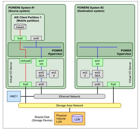
Figure 11-14 Basic virtual Fibre Channel infrastructure before migration
