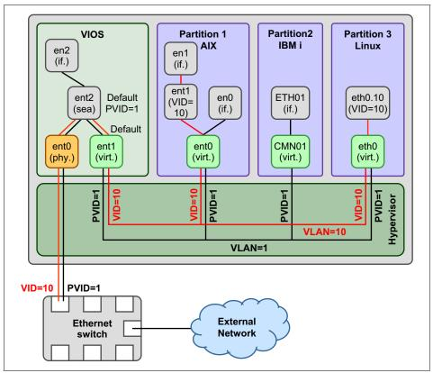
Figure 10-23 VLAN configuration example
