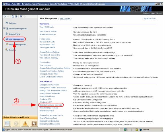
Figure 17-2 HMC option for remote command execution
