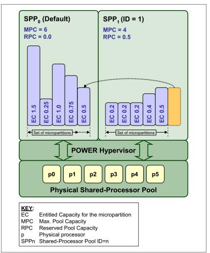
Figure 8-3 Example of micro-partition moving between Shared-Processor Pools
