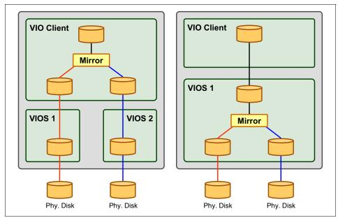
Figure 4-16 Implementing mirroring at client or server level
