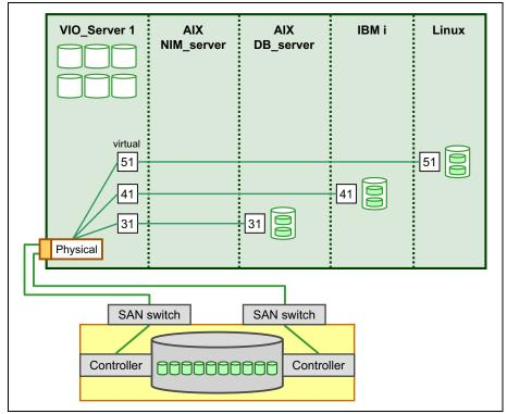
Figure 16-14 depicts the setup of Virtual Fibre Channel described in this section.
