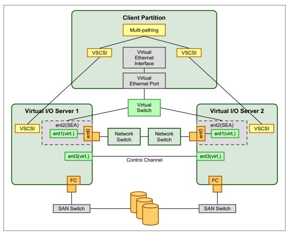
Figure 10-1 Redundant Virtual I/O Servers before maintenance
