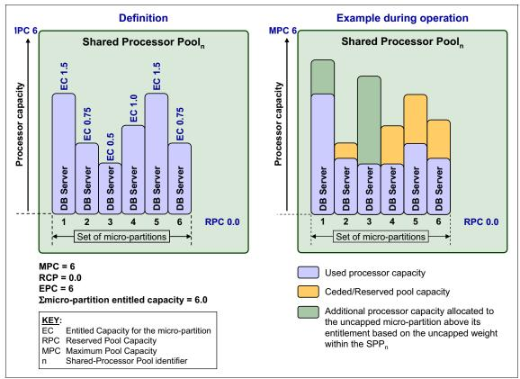
Figure 8-7 Capped Shared-Processor Pool offering database services
