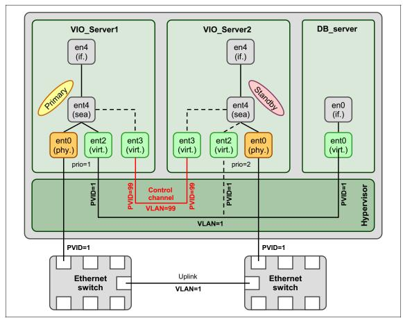
Figure 16-73 Highly available Shared Ethernet Adapter setup
