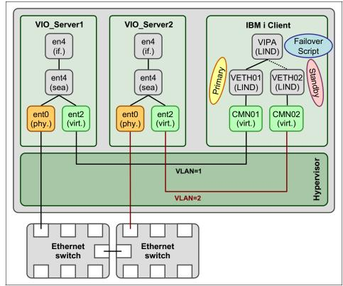
Figure 16-78 VIPA failover configuration for IBM i client
