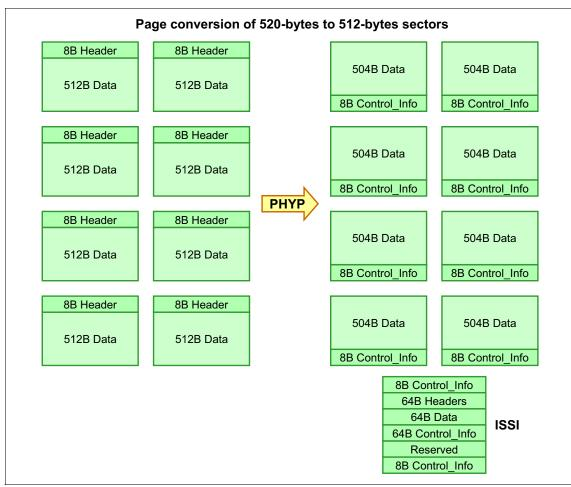
Figure 4-10 Page conversion of 520-bytes to 512-bytes sectors
