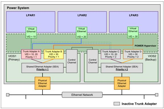
Figure 10-28 shows a basic SEA failover configuration. All network packets of all Virtual I/O clients are bridged by the primary Virtual I/O Server.
