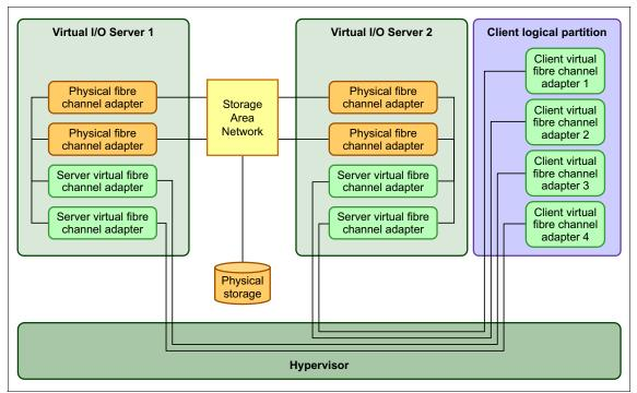
Figure 4-5 Host bus adapter and Virtual I/O Server failover
