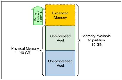
Figure E-1 shows an example partition that has Active Memory Expansion enabled.
