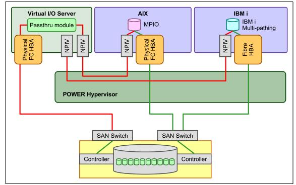
Figure 10-9 Heterogeneous multipathing configuration with Virtual Fibre Channel
