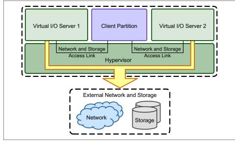
Figure 7-1 Sample for dual Virtual I/O Servers architecture
