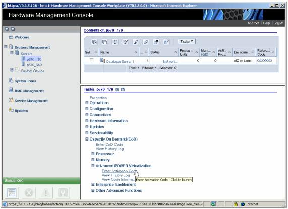
Figure 1-2 HMC window to activate PowerVM feature
