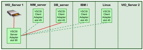
Figure 16-25 SCSI setup for shared optical device
