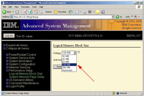
Figure 17-4 Checking and changing LMB size with ASMI
