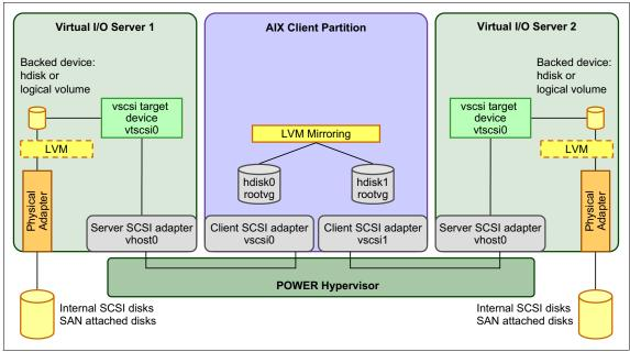
Figure 10-15 shows the best way for mirroring the virtual disks on the client partitions.
