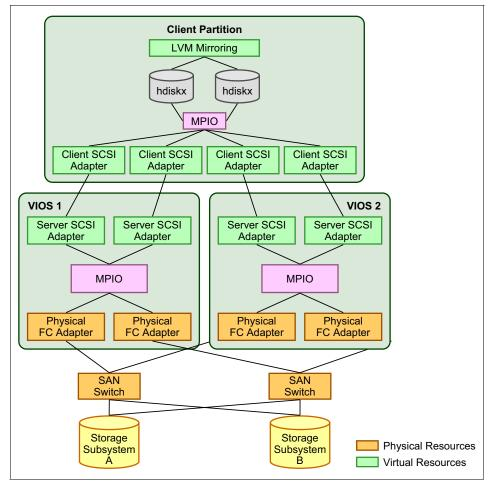
Figure 10-12 LVM mirroring with two storage subsystems
