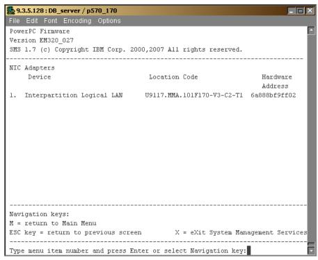
Figure 13-18 Selecting the network adapter for remote IPL
