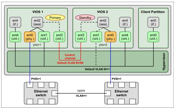
Figure 10-26 shows an alternative setup where the IP address of the Virtual I/O Servers is configured on a separate physical Ethernet adapter.
