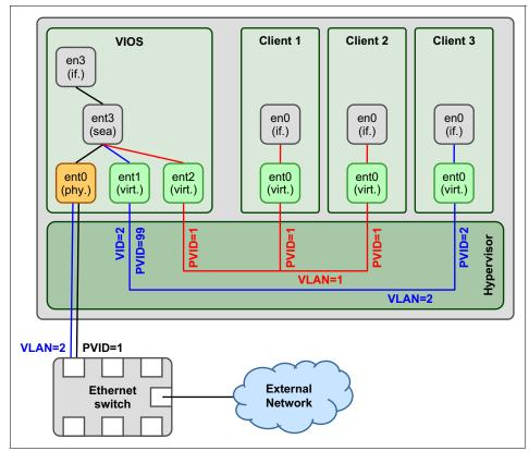
Figure 10-22 Shared Ethernet Adapter
