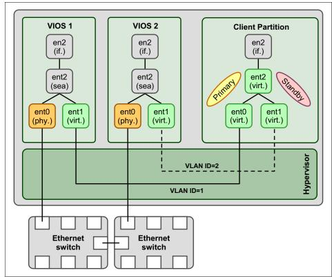
Figure 10-27 Network redundancy using two Virtual I/O Servers and NIB
