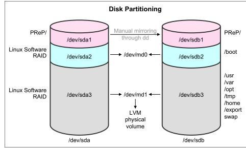
Figure 16-67 shows a generic disk partitioning configuration for Linux.
