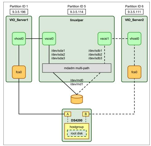
Figure 16-66 Linux client partition using mirroring with mdadm
