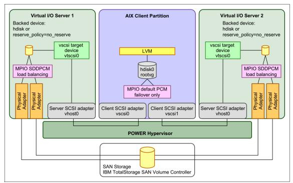
Figure 10-18 Configuration for IBM TotalStorage SAN Volume Controller
