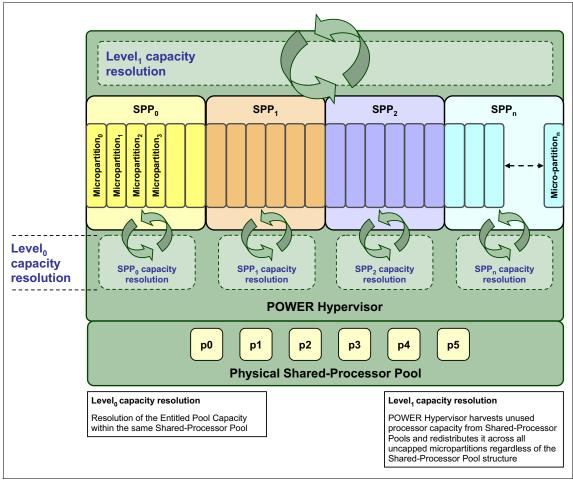
Figure 8-4 The two levels of unused capacity redistribution
