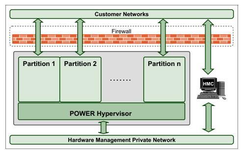
Figure 11-1 Network connections sample for Dynamic Logical Partitioning
