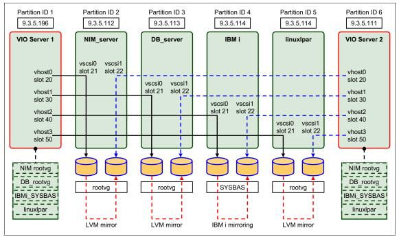
Figure 16-39 Redundant Virtual I/O Server client mirroring scenario
