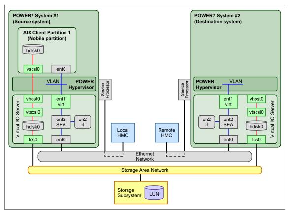
Figure 11-18 displays the Live Partition Mobility infrastructure involving the two remote HMCs and their respective managed systems.
