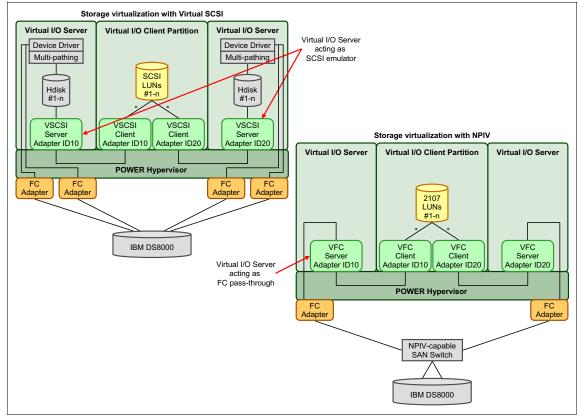
Figure 10-6 Comparing virtual SCSI and Virtual Fibre Channel
