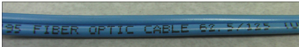
Figure 1-11 Blue 62.5 micron MMF cable
