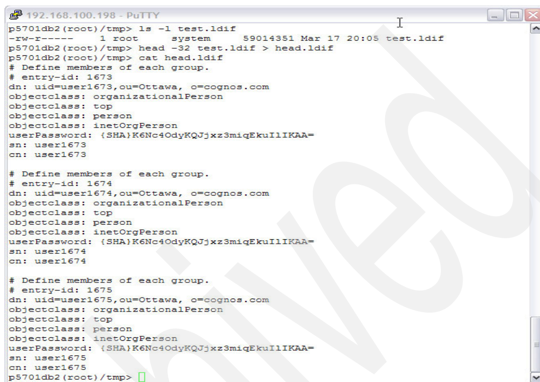
Figure 7-4 Extracting the top three user IDs in an LDIF file
