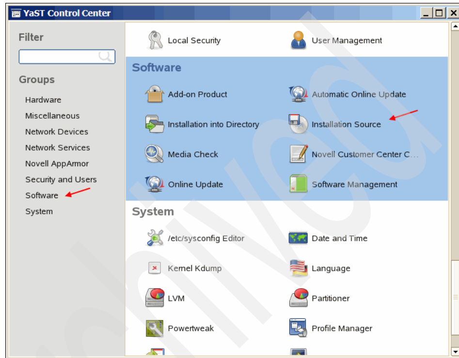
Figure 4-3 Adding an installation source on YaST
