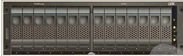
Figure 2-54 EXN1000 expansion unit
