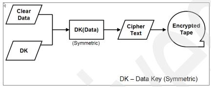
Figure 9-6 LTO4 encryption process
