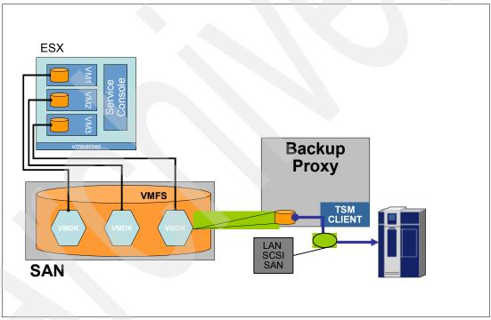
Figure 17-1 VMware consolidated backup in file-level mode
