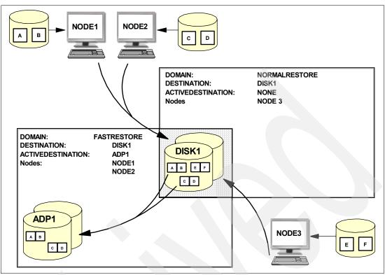
Figure 7-2 Data flow with ACTIVEDESTINATION option
