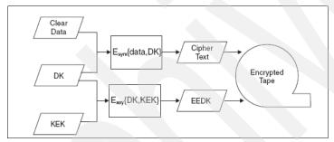
Figure 9-5 TS1120 encryption process
