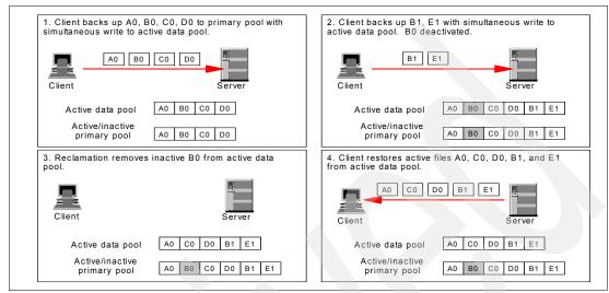
Figure 7-5 Collocation of active data using ADP
