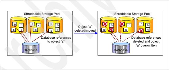
Figure 8-1 How data shredding works
