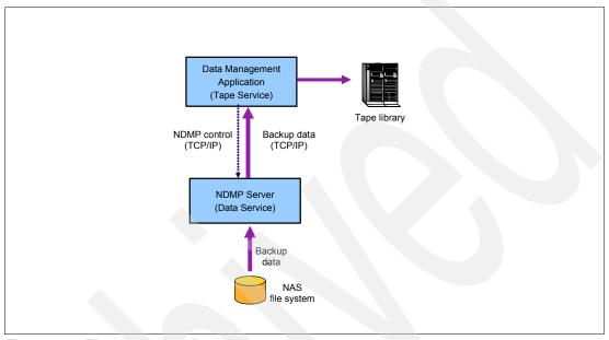
Figure 10-2 Filer-to-server configuration
