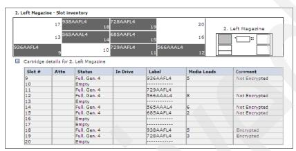
Figure 9-4 Inventory details confirming tape is encrypted in TS3200
