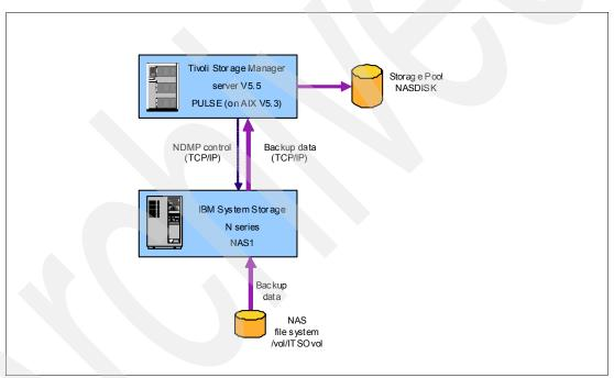
Figure 10-6 Filer-to-server configuration
