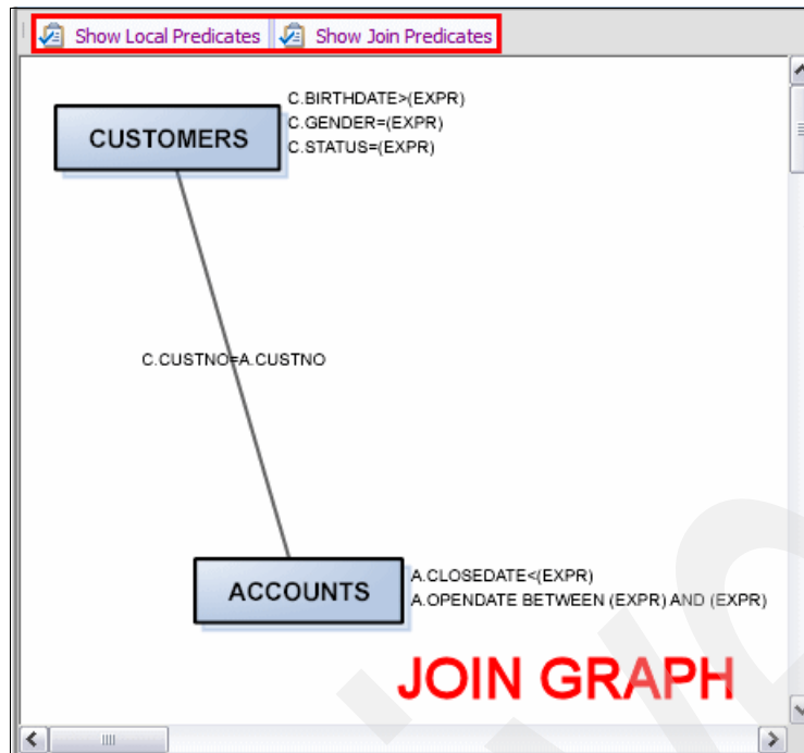
Figure 8-34 Join graph with added predicates
