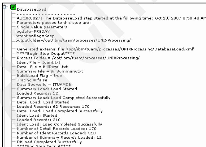
Figure 5-15 Results of the DatabaseLoad step of the LoadUNIX job
