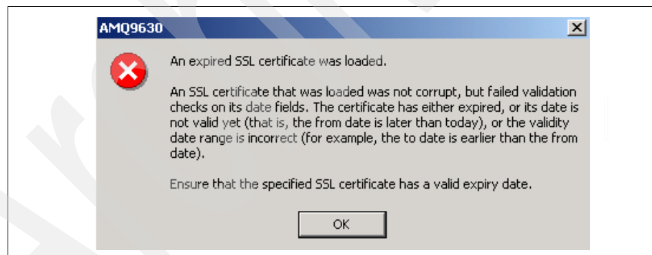
Figure 3-10 SSL certificate date inconsistency error
