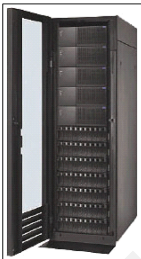
Figure 2-12 A rack with FD4500 servers and disk expansion units
