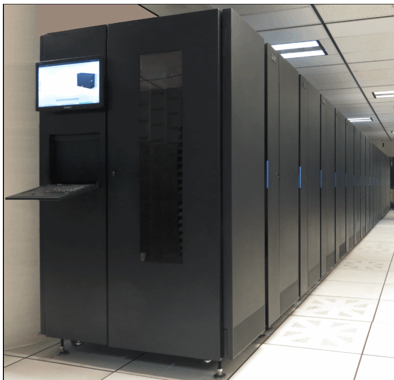
Figure 8-18 Maximum TS4500 tape library configuration with 18 frames
